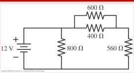
Find the current through and the potential difference across each of the four resistors in the circuit above.
