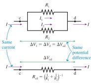
(b) An equivalent resistor
