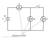
• When the switch is open, A and B are in series with  $R_{eq} = 2R$  and current is
