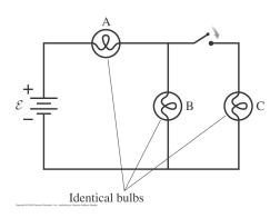
What happens to the brightness of A and B when the switch is closed? How does the brightness of C compare to that of A and B?
