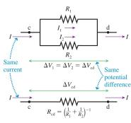
(b) An equivalent resistor
