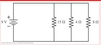
Three resistors are connected in parallel to a 9V battery. Find the potential difference across and the current through each resistor. (Note: assume an ideal battery and ideal wires)
