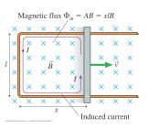
The flux through the loop increases as the wire moves, so
