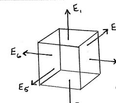
Choose a Gaussian surface in the shape of a cube. The E3 electric field at each face will have the same magnitude and be perpendicular to that face.
