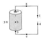
$$\Delta V_{12} = \begin{array}{ccc} \mathbf{OV} & \Delta V_{23} = \begin{array}{ccc} \mathbf{3V} \\ \Delta V_{34} = \begin{array}{ccc} \mathbf{OV} & \Delta V_{14} = \begin{array}{ccc} \mathbf{3V} \\ \mathbf{\vec{E}_a} \end{array}$$
