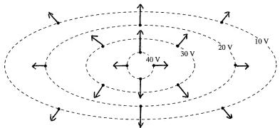
7. Draw the electric field vectors at the dots on this contour map. The length of each vector should be proportional to the field strength at that point.
