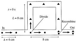
Constructively. The path length difference is an integer multiple of the wavelength. The wave crest positions are the same at the output
