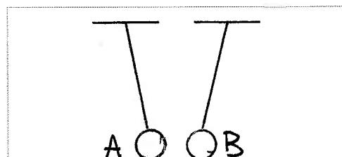
d. Both are charged by a plastic rod, but ball A is charged more than ball B.
