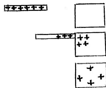
12. A lightweight, positively charged ball and a neutral rod hang by threads. They are close but not touching. A positively charged glass rod touches the hanging rod on the end opposite the ball, then the rod is removed.
