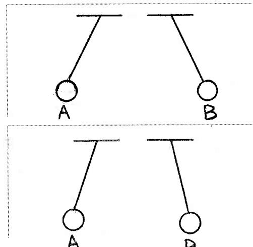
c. Ball A is touched by a plastic rod that was rubbed with wool and ball B is touched by a glass rod that was rubbed with silk.
