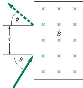
As you can see from the figure, lines drawn perpendicular to the trajectory at entry and exit form an isosceles right triangle. The Trajectory is symmetric so  $r^2 + r^2 = d^2$ .
