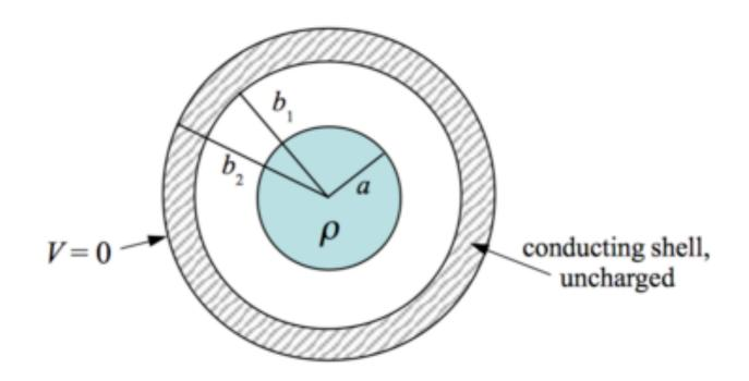
Consider a non-conducting <u>cylinder</u> of infinite length and radius a, which carries a volume charge density p. Surrounding this object is an uncharged conducting cylindrica shell. The metal tube is also of infinite length, and its inner and outer radii are b<sub>1</sub> and b<sub>2</sub> respectively. In this problem, we will define the potential to be zero at the outer surface of the conducting shell.
