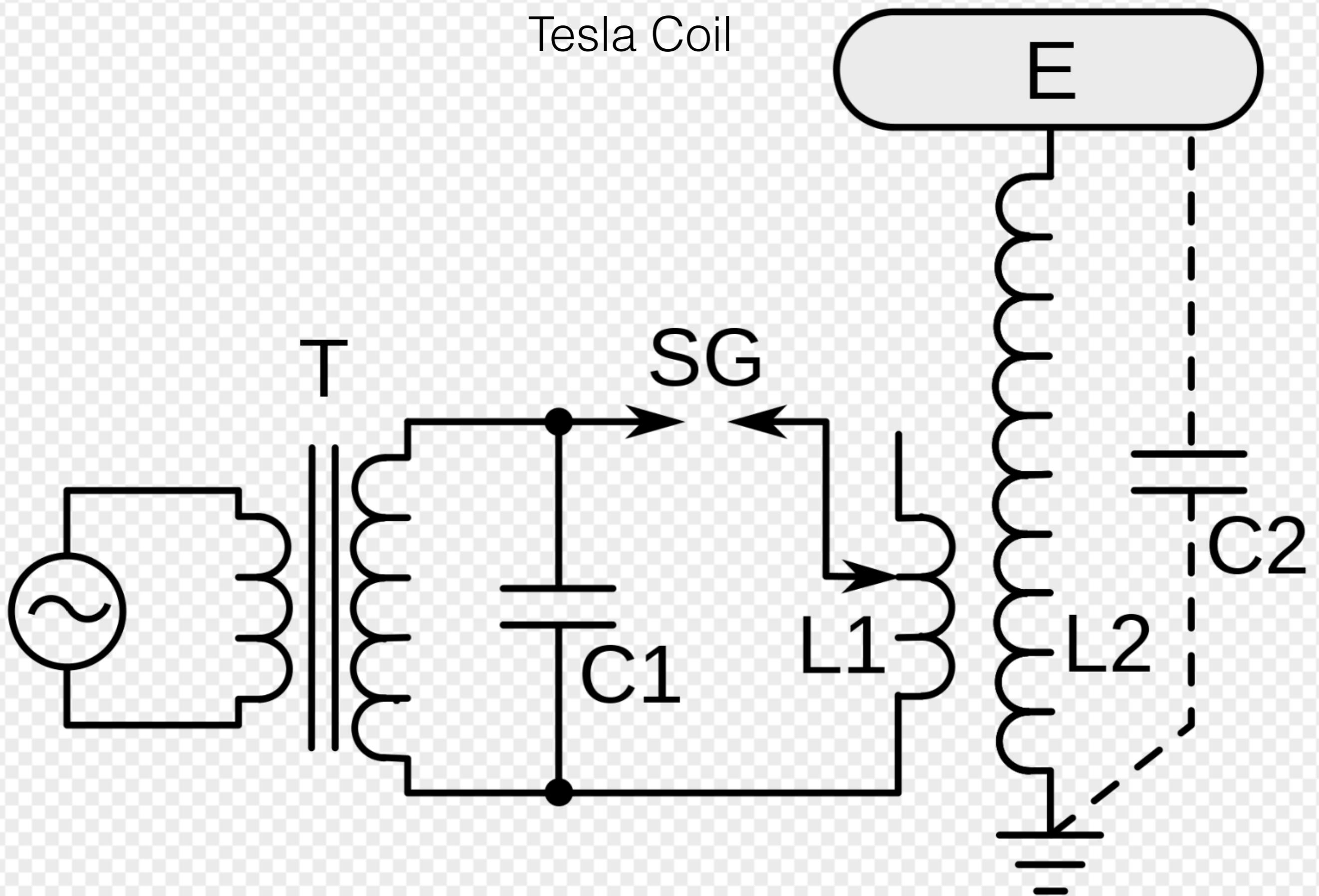
Unipolar Tesla coil circuit.  $C_2$  is not an actual capacitor but represents the parasitic capacitance of the secondary windings  $L_2$ , plus the capacitance to ground of the toroid electrode  $E$ .
