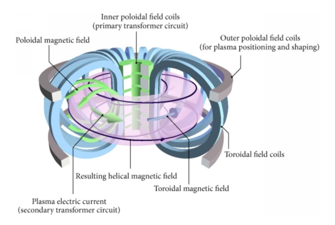
Tokamak: Nuclear Fusion Reactor
