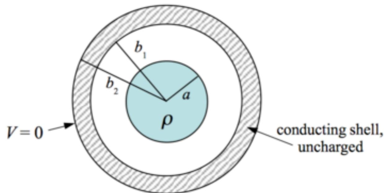
Consider a non-conducting cylinder of infinite length and radius  $a$ , which carries a volume charge density  $\rho$ . Surrounding this object is an uncharged conducting cylindrical shell. The metal tube is also of infinite length, and its inner and outer radii are  $b_1$  and  $b_2$  respectively. In this problem, we will define the potential to be zero at the outer surface of the conducting shell.
