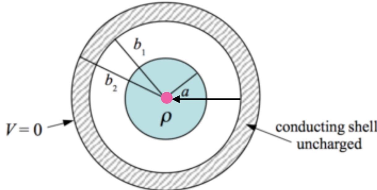
What is the electric potential at the center of the non-conducting cylinder?
