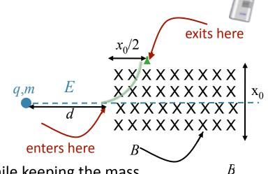
Suppose the charge of the particle is doubled (Q = 2q), while keeping the mass constant. How does the path of the particle change?
