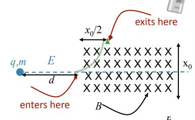
Suppose the charge of the particle is doubled (Q = 2q), while keeping the mass constant. How does the path of the particle change?
