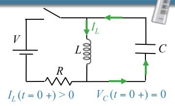
What is the direction of the current immediately after the switch is opened?
