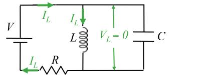
The switch in the circuit shown has been closed for a long time. At t=0, the switch is opened.
