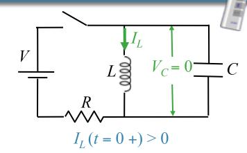
The energy stored in the capacitor immediately after the switch is opened is zero.
