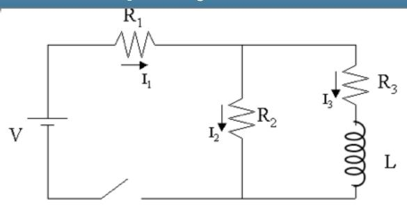
At what time, does the current through the inductor  $I_3$  reach a value that is 63% of its maximum value?
