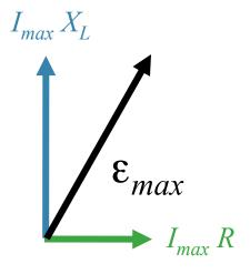
The voltages across the resistor and the inductor are
