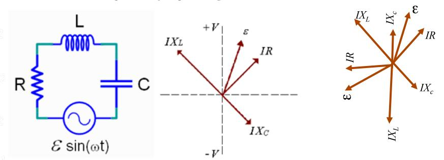
When the capacitor is fully charged, what is the magnitude of the voltage across the inductor?
