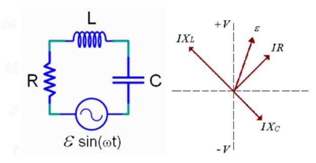
The vertical axis of the phasor diagram represents voltage. When the current through the circuit is maximum, what is the potential difference across the inductor?
