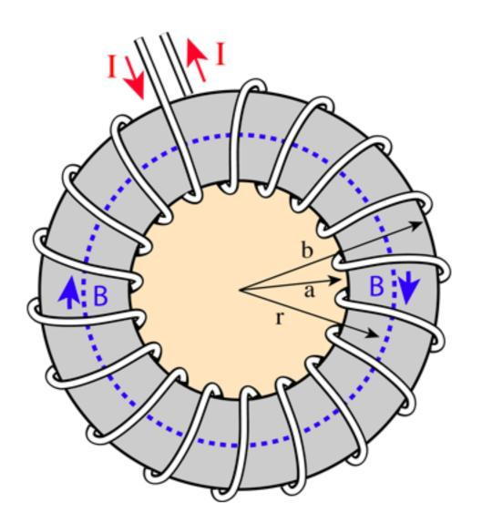
Air-core toroidal inductor with an inductance of 1 mH.
