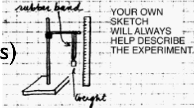
I put different masses on the end of the rubber band and recorded the position of the top of the hook that holds the weight
