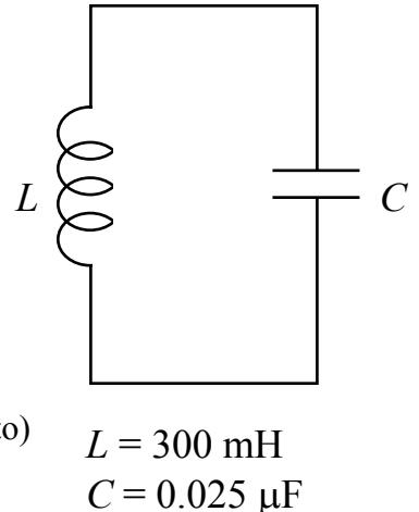
**(a) What is the angular frequency  $\omega_0$  of the current maintained by the circuit? What is the linear frequency  $f_0$ ?**
