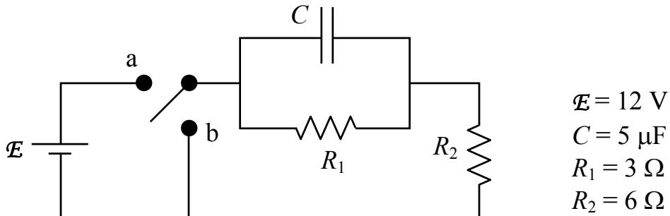
(a) At  $t = 0+$ , immediately after the switch is thrown to position a, what are the currents  $I_1$  and  $I_2$  across the two resistors?
