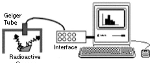
Figure 2-1: A Radiation Monitoring System
