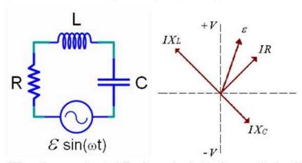
When the capacitor is fully charged, what is the magnitude of the voltage across the inductor?
