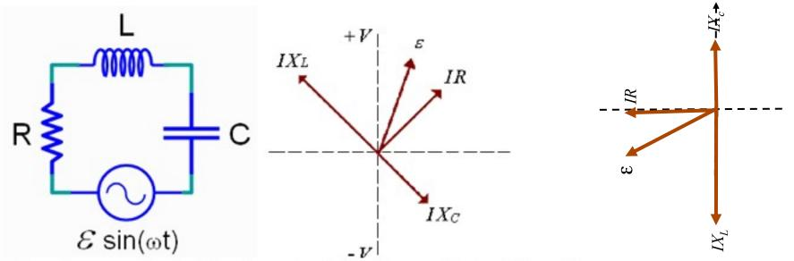
12) When the voltage across the capacitor is at its positive maximum,  $V_C = +V_{Cmax}$ , what is the voltage across the inductor?
