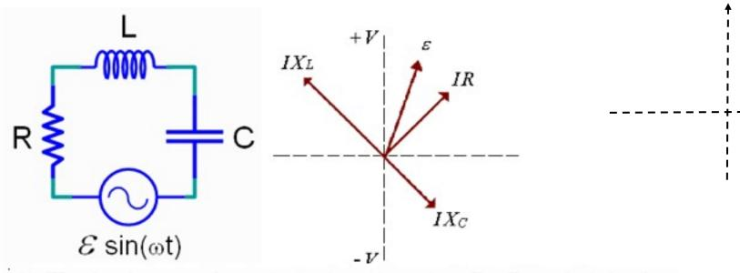
12) When the voltage across the capacitor is at its positive maximum,  $V_C = +V_{Cmax}$ , what is the voltage across the inductor?
