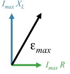
The voltages across the resistor and the inductor are \_\_\_\_\_
