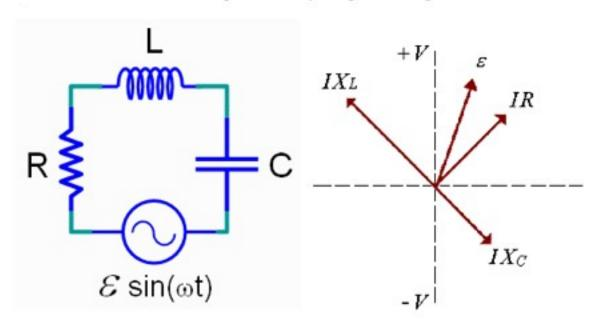
The vertical axis of the phasor diagram represents voltage. When the current through the circuit is maximum, what is the potential difference across the inductor?
