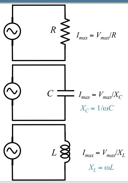
$V_R$  in phase with IBecause resistors are simple
