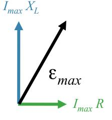
The voltages across the resistor and generator are \_\_\_\_\_
