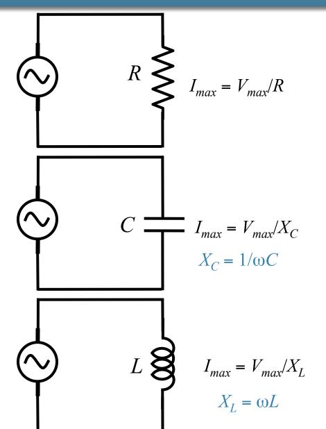
$V_R$  in phase with IBecause resistors are simple
