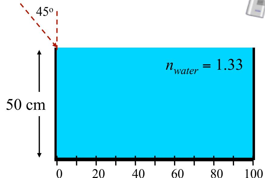
If you shine a laser into the tank at an angle of  $45^\circ$ , what is the refracted angle  $\theta_R$  in the water ?
