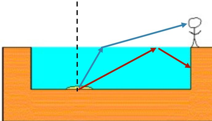
Can the person standing on the edge of the pool be prevented from seeing the light by total internal reflection at the water-air surface?
