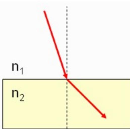
Compare the indexes of refraction in the two mediums.
