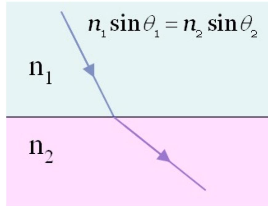
Light travelling through a medium with index of refraction  $n_1$  is refracted as it enters a medium with index of refraction  $n_2$  as shown in the figure to the right. Based on this figure what can you infer about the index of refraction of the two materials?
