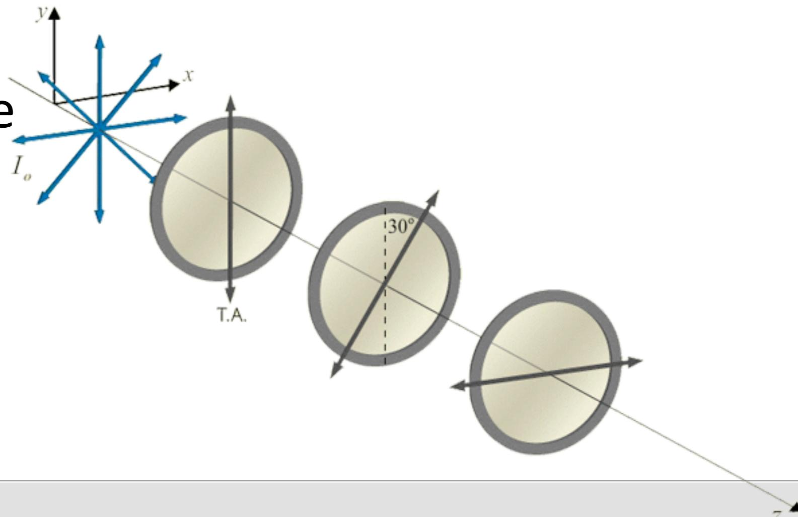
Unpolarized light of intensity  $I_0$  is incident on a set of three linear polarizers oriented at  $0^\circ$ ,  $30^\circ$  and  $90^\circ$  with respect to vertical as shown. The intensity of the light after passing through all three polarizers is  $I_{\text{final}}$ .
