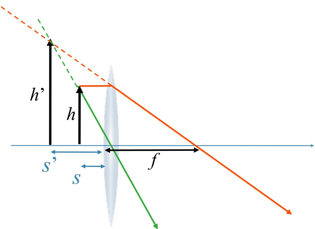
A magnifying glass is used to read the fine print on a document. The focal length of the lens is 10mm.
