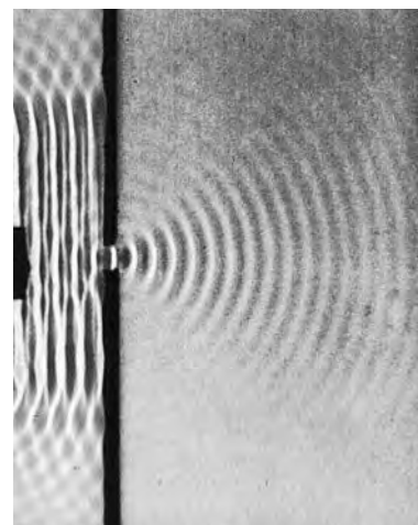
FIGURE 33-6 Plane water waves in a ripple tank encountering a barrier that has a small opening. The waves to the right of the barrier are circular waves that are concentric about the opening, just as if there were a point source at the opening. (From PSSC Physics , 2nd Edition, 1965. D. C. Heath & Co. and Education Development Center, Newton MA.)
