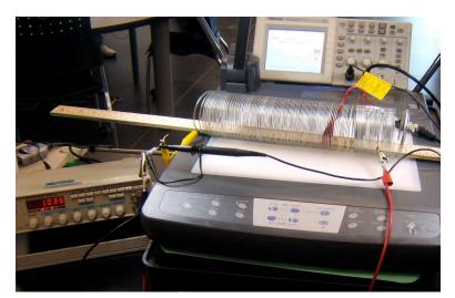
I managed to set up the complete apparatus on the AV stand so that the Elmo could display the apparatus on the projectors. The oscilloscope is perched (precariously) on the back of the stand so that the camera could be tilted to display the oscilloscope screen to the class. The pick-up coil is inside the slinky.
