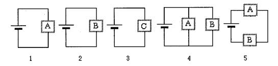
a) For each of the circuits 1 through 5, sketch below a standard circuit diagram showing all the bulbs in the circuit. In each diagram number the bulbs and describe which bulbs or combination of bulbs are in series and parallel connections with each other.
