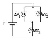
(c) Develop mathematical equations that express the relationships between the emf of the battery (assuming it has no internal resistance) and the potential differences  $\Delta V_1$ ,  $\Delta V_2$ , and  $\Delta V_3$  for the circuit shown.
