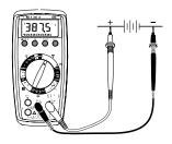
A Digital Multimeter (DMM) used as a voltmeter and connected to a battery.
