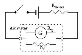
Figure 25-7: Ammeter in series with a resistor and battery.
