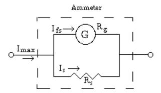
**Figure 25-6**: Wiring an ammeter unit using a galvanometer and shunt resistor.
