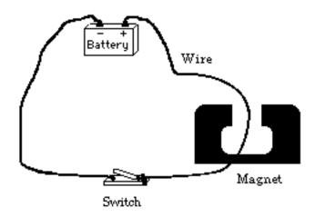
Figure 25-3: Wire that can carry current in a magnetic field.
