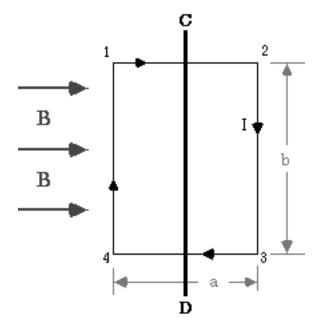
**Figure 25-4**: A Loop of wire of dimensions a,b in a magnetic field of magnitude *B*.
