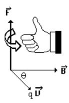
**Figure 25-2**: Use of the Right Hand Rule to Find the Direction of a Magnetic Force Exerted on a Moving Charge
