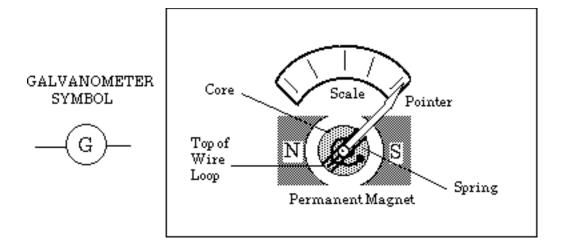
Figure 25-5: The Guts of a Typical Galvanometer
