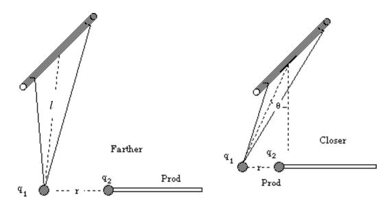
Using the laws of mechanics, it is possible to determine the relationship between the Coulomb force on the small sphere and the angle through which it rises above a vertical line. Thus, you should be able to measure the Coulomb force on  $q_1$  as a function of the distance between  $q_1$  and  $q_2$ .
