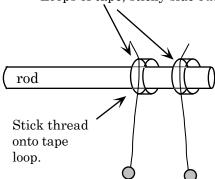
You can suspend the balls from a rod by wrapping two loops of tape around the rod with the sticky sides of the tape facing out. Then just push the thread onto the tape's adhesive. The distance between balls can be changed by sliding a loop left or right. The height of the ball can be adjusted by carefully rotating the tape loop
