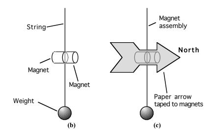
**Figure 26-1: (b)** Alternative to compass. A string is clamped between two small, cylindrical neodynium magnets. A small weight is suspended from the string. **(c)** A paper arrow is taped to the magnets.
