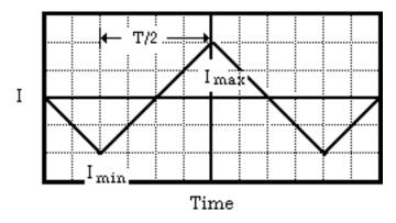
**Figure 26-10**: A graph of current vs. time in the field coil when a triangle wave form is fed into a field coil.
