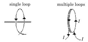
**Figure 26-6:** A wire loop carrying a current *I*.
