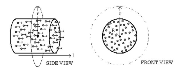
**Figure 26-4:** An imaginary circular Ampèrian loop of radius r constructed outside a conductor of radius R which carries a current I. The moving charges are indicated by the small gray dots.
