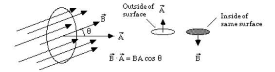
**Figure 26-8**: Magnetic flux through an area A is the dot product of the magnetic field vector and the vector normal to the area.
