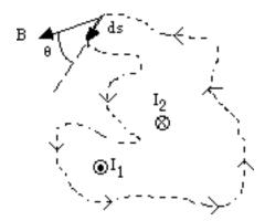
**Figure 26-3:** A General Ampèrian Loop w/ Net Current  $I = I_1 - I_2$ . The dotted line represents one of an infinite number of possible closed loops that enclose the two wires carrying currents  $I_1$  and  $I_2$ . **Note**: The dotted loop represents an imaginary path, not a wire!
