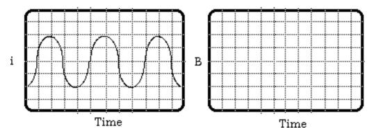
(b) Set the data logger software to a high data collection rate. We'd suggest 1000 data points per second. Set the magnetic field sensor to maximum sensitivity. The Hall effect sensor reacts to a magnetic field that is *perpendicular* to its flat area. How should the sensor be placed relative to the orientation of a wire inside an electric blanket to get the maximum B-field measurement? Draw a sketch, if needed.
