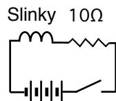
3. The  $10\Omega$  resistor serves to limit the current and can be used to monitor the current with a voltage probe. ( $I = V/R$ ) The slinky itself has a resistance of several ohms and you should measure it.
