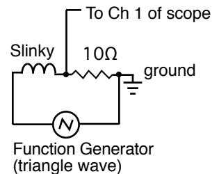
2. Use oscilloscope channel 1 to monitor the voltage across the  $10\ \Omega$  resistor. Clip the  $x10$  probe to the resistor on the end closest to the slinky. The ground of the probe should be the same as that of the function generator, i.e., the other end of the resistor.
