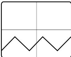
4. Adjust the function generator to make a triangle wave of 1 kHz at maximum amplitude. Display the ch 1 signal, the voltage across the  $10\ \Omega$  resistor, on the bottom half of the oscilloscope screen with a time scale that shows about two or three complete cycles. The trigger source should always be ch 1.
