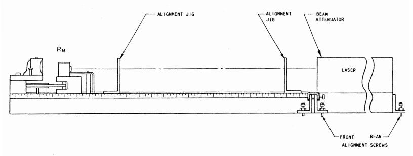
The laser must be aligned so the beam strikes the center of the rotating mirror (R<sub>m</sub>). Two alignment jigs are provided for this purpose. Place one jig at each end of the optical bench as shown above, with the edges flush against the fence of the bench. When properly placed, the holes in the jigs define a straight line that is parallel to the axis of the optical bench.
