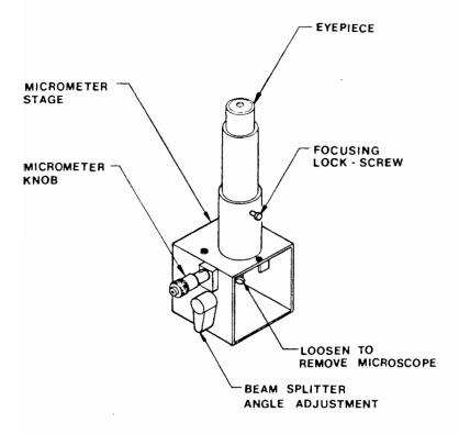
The 90X microscope is mounted on a micrometer stage for precise measurements of the image point displacement. Measurements are most easily made by visually centering the image point on the microscope cross-hairs. The micrometer graduations then permit the displacement to be resolved to within 0.005 mm.
