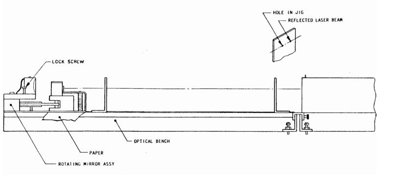
5. Align the Rotating Mirror: R<sub>m</sub> must be aligned so its axis of rotation is vertical and perpendicular to the laser beam. Rotate R<sub>m</sub> so that the laser beam reflects back toward the hole in the alignment jig. Be sure to use the silvered side of the mirror as the reflecting surface, and tighten the lock-screw on the rotating mirror assembly just enough so R<sub>m</sub> holds its position as you adjust its rotation.
