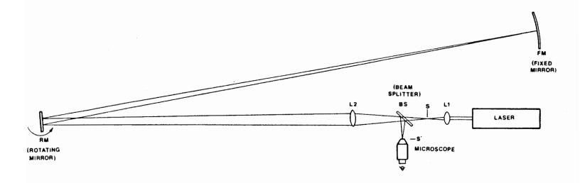
In this experiment you will use a method that is basically the same as that developed by Foucault in 1862. A diagram of the experimental setup is shown above.
