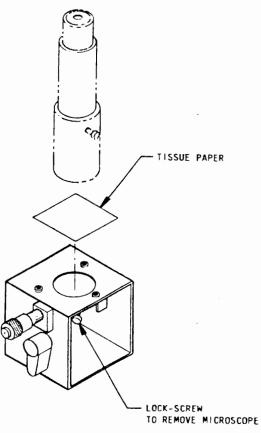
If you still can not find the point image, loosen the screw that attaches the microscope to the micrometer stage. As shown above, remove the microscope and place a piece of tissue paper over the hole in the stage to locate the beam. Adjust the beam splitter angle and the micrometer stage position to center the point
