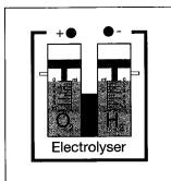
An electrolyser contains an electrolyte and two electrodes (the positive anode and the negative cathode). When a voltage is applied, the ions (charge carriers) in the electrolyte will be attracted to the electrodes and a current flows. However the voltage has to be high enough (enough energy) to 'split the water' into its ions before a current will flow – the decomposition voltage.
