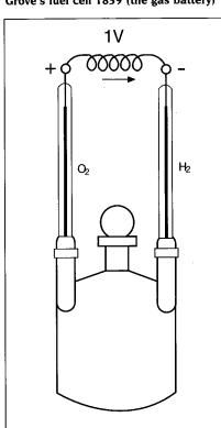
around 1 volt. It seemed that the hydrogen molecules were returning to the electrode and giving up their electrons. These electrons were travelling round the circuit to the positive electrode and there they were ionising the oxygen. On the way round the circuit the electrons could power electrical apparatus.
