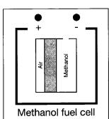
A direct methanol fuel cell produces an emf by using methanol directly as a fuel and oxidising it to carbon dioxide. A fuel cell will provide energy so long as liquid methanol is supplied to it. This type of fuel cell is favoured for many applications as carrying methanol in a fuel tank is much more straight forward than carrying hydrogen.
