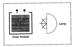
A solar cell is a specially designed semiconductor diode which generates an e.m.f. when exposed to light. The solar cell absorbs light energy and converts it to electrical energy so the amount of light falling on the solar cell will affect the current output.
