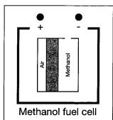
A direct methanol fuel cell produces an emf by using methanol as a fuel and oxidising it directly to carbon dioxide. The fuel cell will provide energy so long as liquid methanol is supplied to it. This type of fuel cell is favoured for many applications as carrying methanol in a fuel tank is much more straight forward than carrying hydrogen.
