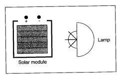
A solar cell is a specially designed semiconductor diode which generates an e.m.f. when exposed to light. The solar cell absorbs light energy and converts it to electrical energy so the amount of light falling on the solar cell will affect the current output.
