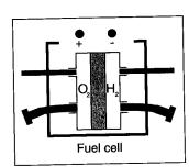
A hydrogen fuel cell produces an emf by combining hydrogen and oxygen chemically. A conventional battery supplies electrical energy in the same way except that the reactants (for example nickel oxyhydroxide and cadmium) are eventually used up and the battery has to be disposed of or recharged. A fuel cell will provide energy so long as hydrogen and oxygen are supplied to it. The current and voltage output will depend upon the load applied
