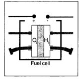
The dismantlable fuel cell works as a typical hydrogen fuel cell. It produces an emf by combining the hydrogen and oxygen from electrolysis chemically. It will provide energy so long as hydrogen and oxygen are supplied to it.
