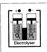
The electrolyser-fuel cell system is a convenient way of storing solar generated electricity. The electrolyser produces supplies of hydrogen and oxygen which can be fed to the fuel cell when power is required. As with any power conversion there are energy losses - less electricity is supplied than was first generated. The efficiency also varies according to the load resistor through which the fuel cell is having to drive the current.
