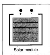
A solar cell will not produce an e.m.f. itself unless it is irradiated. A power supply can make a current flow through a non-irradiated solar cell and this current will vary as the applied e.m.f. is changed. The characteristic curve, a plot of I against V, of the solar cell will show whether it is acting as a diode when not irradiated.
