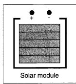
A solar cell is a specially designed semiconductor diode which generates an e.m.f. when exposed to light. The solar cell absorbs light energy and converts it to electrical energy so the amount of light falling on the solar cell will affect the current output. A solar module is a number of solar cells connected in series.
