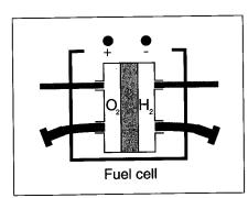
A hydrogen fuel cell produces an emf by combining hydrogen and oxygen chemically. A conventional battery supplies electrical energy in the same way except that the reactants (for example nickel oxyhydroxide and cadmium) are eventually used up and the battery has to be disposed of or recharged.
