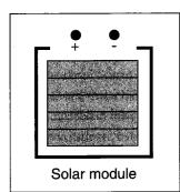
A solar cell will not produce an e.m.f. itself unless it is irradiated. A power supply can make a current flow through a non-irradiated solar cell and this current will vary as the applied e.m.f. is changed. The characteristic curve, a plot of I against V, of the solar cell will show whether it is acting as a diode when not irradiated.
