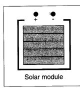
A solar cell is a specially designed semiconductor diode which generates an e.m.f. when exposed to light. It can, therefore, be used as a low voltage D.C. power supply, but only up to a limit. A solar module is a number of solar cells connected in series so that the total e.m.f. obtained is the sum of the individual e.m.f.s. However the current obtained is limited by the internal resistance of each solar cell.
