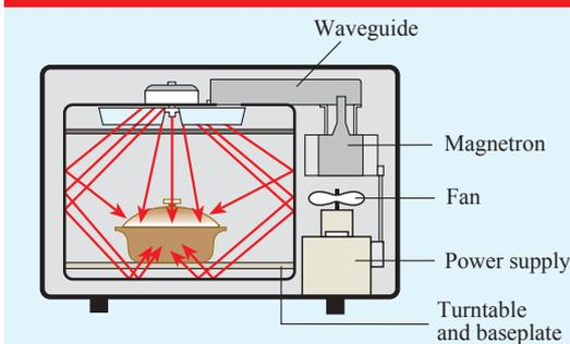
Figure 1. Schematic diagram of a typical microwave oven.
