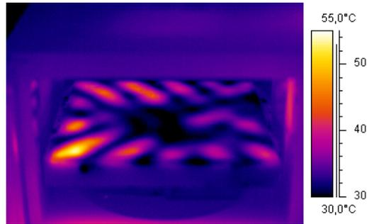
**Figure 4.** Visualization of the horizontal mode structure in a microwave oven using infrared thermal imaging. A glass plate with a thin water film was placed at a height of  $8\text{ cm}$  and heated for  $15\text{ s}$  with a microwave power of  $800\text{ W}$  without using the turntable (for more details on the experiment, see [10]).
