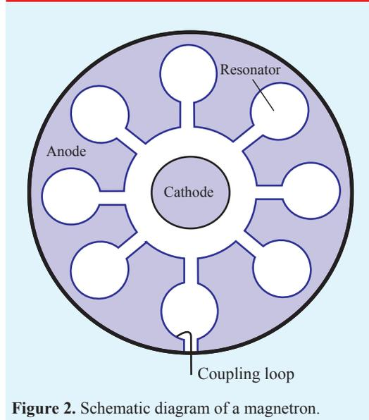
Figure 2. Schematic diagram of a magnetron.
