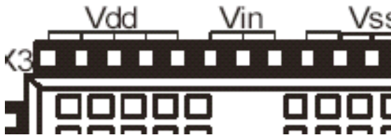
Fig 2: The end of the waffle board has a strip with the following connections: Vdd, regulated 5 V, Vin, unregulated power from the supply or battery, and Vss, ground.
