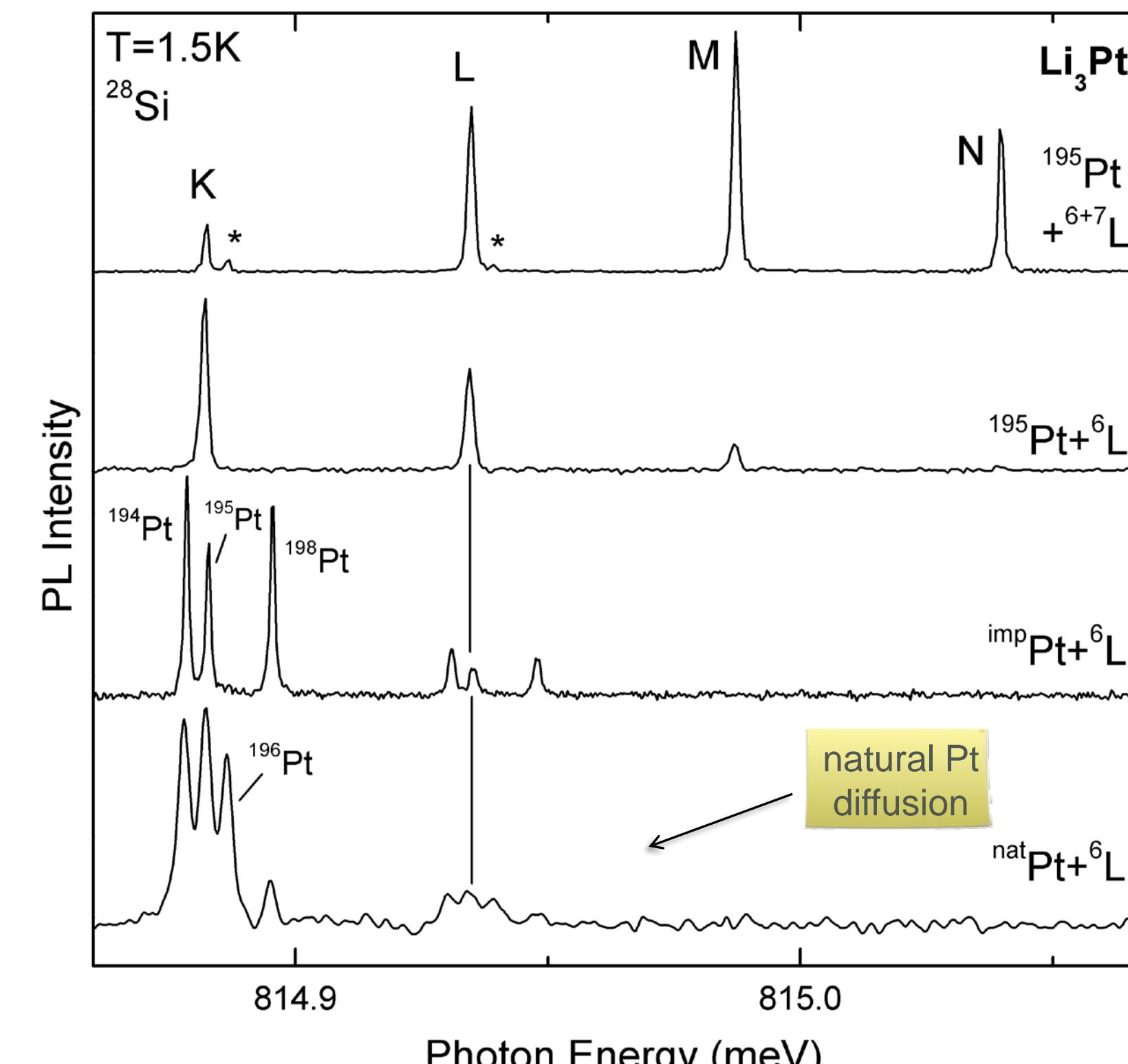
Spectra of the 4-atom  $\text{Cu}_x\text{Li}_{(3-x)}\text{Pt}$  series in  $^{28}\text{Si}$ .
