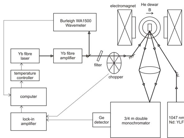
PLE apparatus based on a tuneable single frequency laser source
