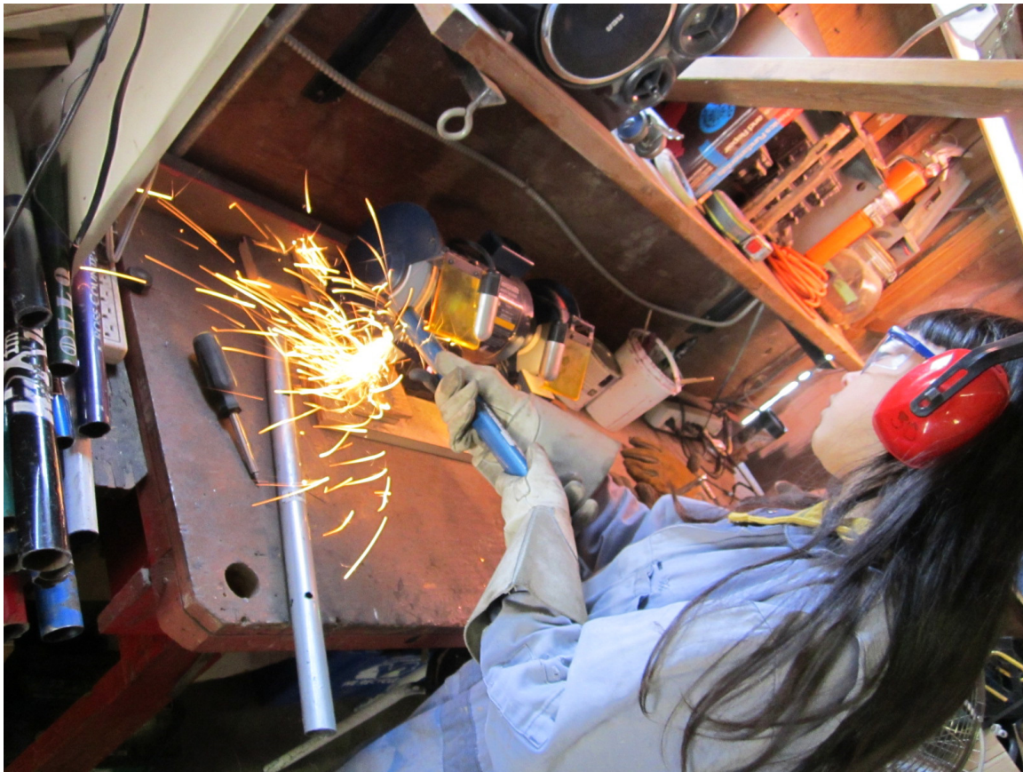
Figure 3.4 Robyn turning discarded bicycle frames into the bars of a gangsa .
