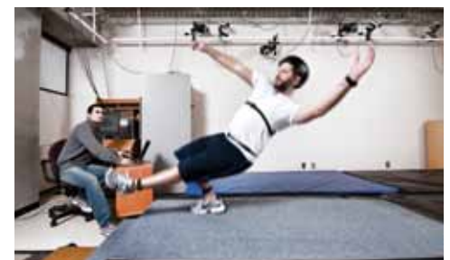
SUB-PROJECT B TIPS trainees Omar Aziz (seated) and Thiago Sarraf conduct experiments in the IPML laboratory to test the ability of wearable sensors to distinguish the cause of falls.
