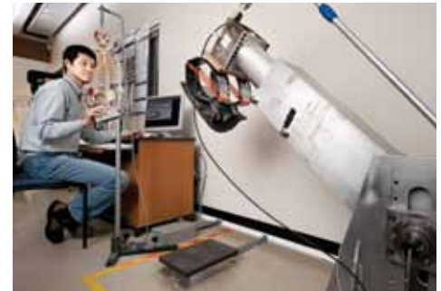
SUB-PROJECT D TIPS trainees measure impact upon simulated hip on floor surface.
