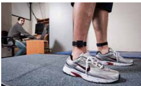
SUB-PROJECT B TIPS trainees Omar Aziz (seated) and Thiago Sarraf conduct experiments in the IPML laboratory to test the ability of wearable sensors to distinguish the cause of falls.
