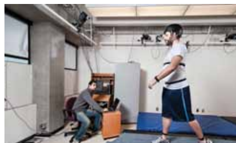
SUB-PROJECT B TIPS trainees Omar Aziz (seated) and Thiago Sarraf conduct experiments in the IPML laboratory to test the ability of wearable sensors to distinguish the cause of falls.
