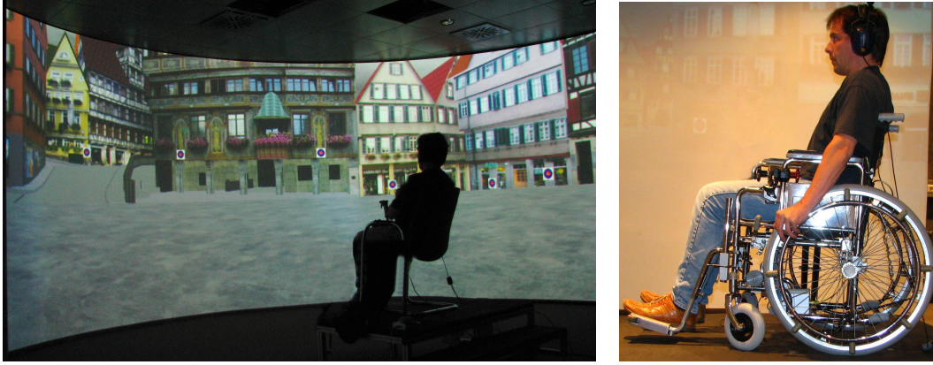
Figure 1: Left: Experimental setup displaying a participant seated in front of the 220^\circ \times 50^\circ cylindrical projection screen showing a view of the 3D model of a market place. Right: Modified wheelchair used as a joystick-like (velocity-control) motion model where participants essentially provide themselves with a minimal motion cueing.
