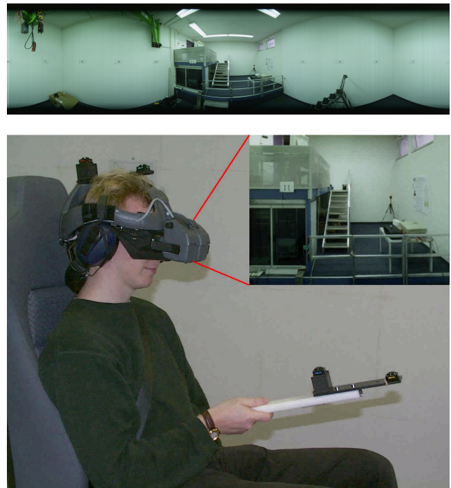
Figure 2: Top: A photorealistic virtual replica of the real Motion-Lab was created from a 360° roundshot (4096 x 1024 pixel) of the real room. Bottom: Participant pointing with the position-tracked pointer and wearing a position-tracked head-mounted display (HMD) and active noise cancellation headphones.
