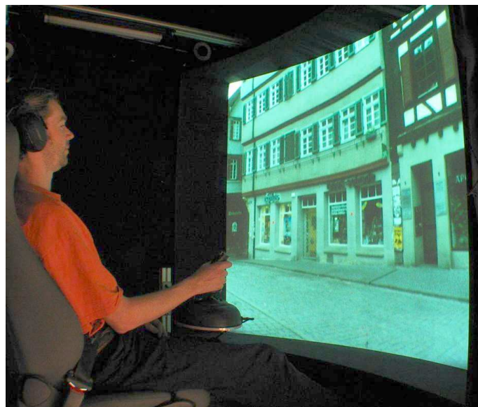
Figure 1: Participant seated in front of curved projection screen displaying a view of the Tübingen market place.
