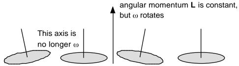
After the rotating disk receives the impulse, it still has a component of  $\omega$  perpendicular to the plane of the disk. But the disk rocks back and forth as well, meaning that there is an oscillating component of  $\omega$  around the 1 and 2 body-fixed axes of the disk. That is, a rocking motion around the 1-axis corresponds to a non-vanishing  $\omega_1$ , such that the vector describing  $\omega$  may have several non-zero components ( $\omega_1$ ,  $\omega_2$ ,  $\omega_3$ ).
