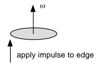
If we hit the disk on its side, generating a torque about the plane, then the plane of the disk will oscillate, as will the corresponding angular velocity vector  $\omega$  (gyroscope demo):
