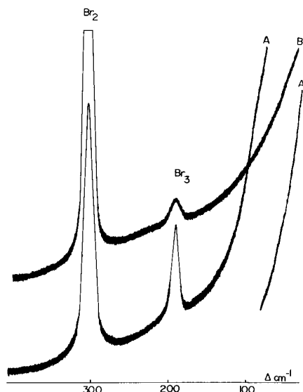
FIG. 2. The matrix Raman spectrum of the products of a \text{Xe}/\text{Br}_2 (50:1) microwave discharge A frozen at 4.2°K; B allowed to diffuse at 35°K for 3 min. and then recooled to 4.2°K.
