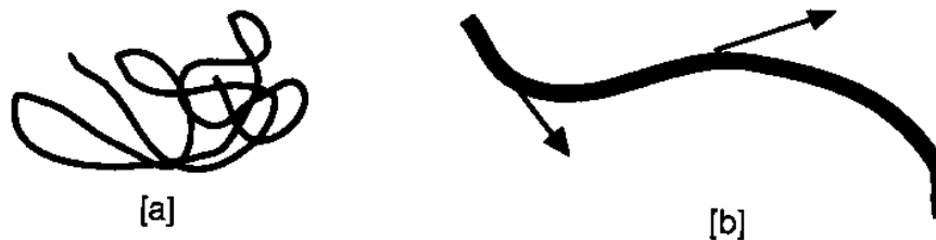
Figure 4. Schematic representation of strings with short [a] and long [b] persistence lengths. The arrows in [b] are about a persistence length apart, as measured along the contour of the string.
