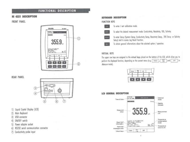
Figure 1. Front panel and keyboard function of HANNA HI 4321 conductivity meter.
