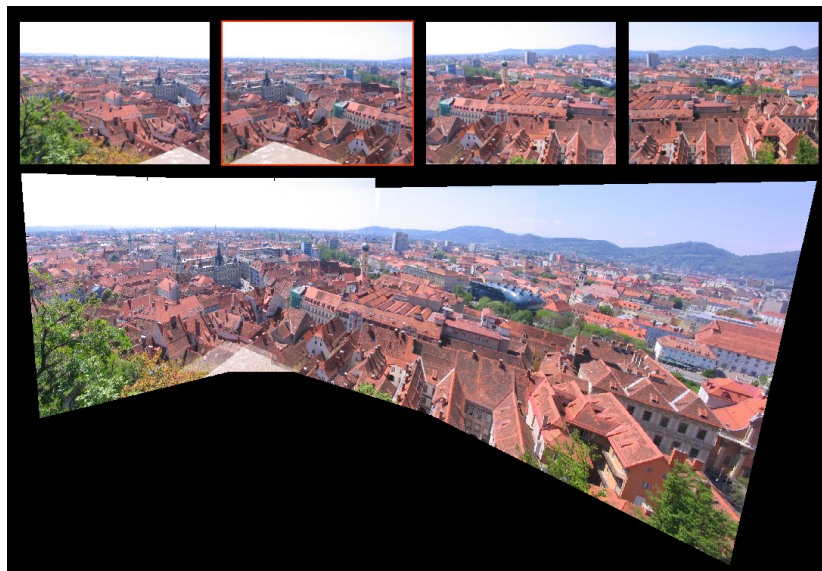
Figure 2: Top: Four images taken from different views at the same location. Bottom: The resultant panorama using the image second from the right (red border) as reference frame.
