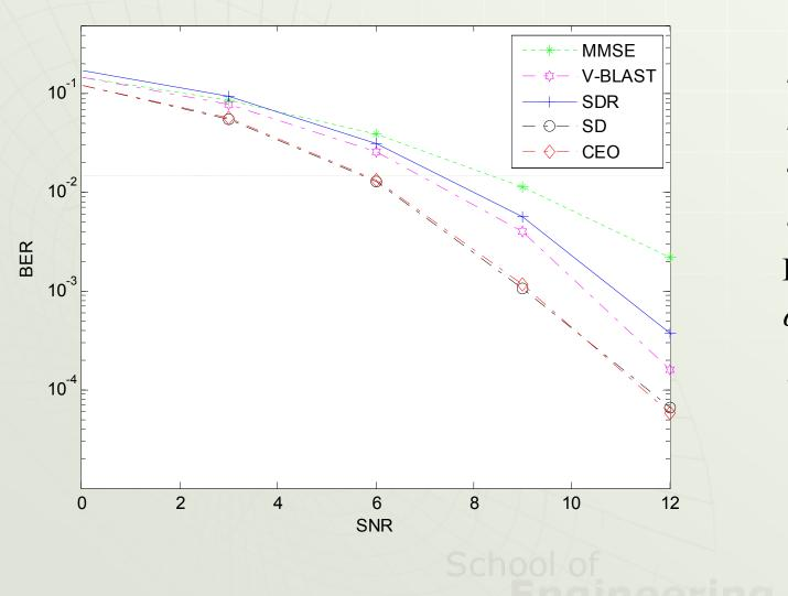
Parameters  $N_T = 4$ K=3 4-QAM  $N_R = 4$  $\Gamma = 100$  $\alpha = 0.7$  $\rho = 0.3$ m = 24
