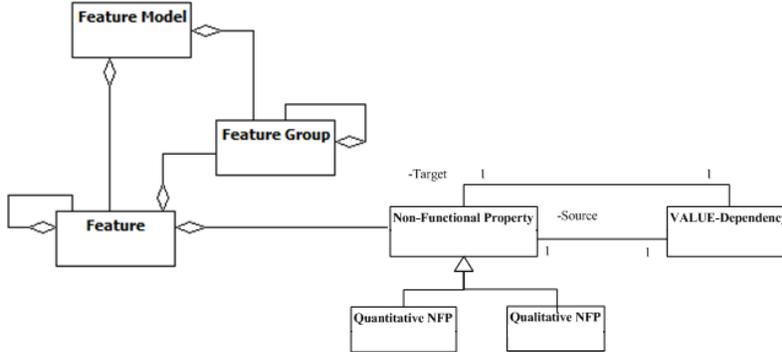
Figure 5: Integration of Feature Model with Non-Functional Property Model
